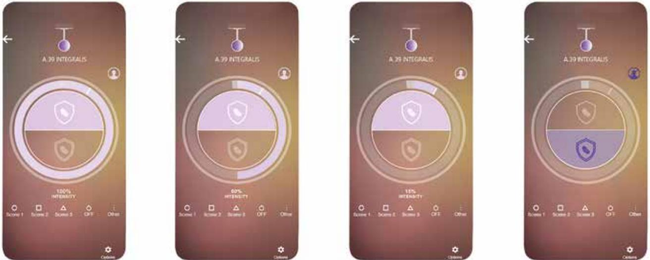
In PURE INTEGRALIS the two activable modes are: MICROBIAL GROWTH CONTROL and ANTIMICROBIAL ACTION. Light intensity can be adjusted (10-100% in PURE INTEGRALIS) in MICROBIAL GROWTH CONTROL only.
